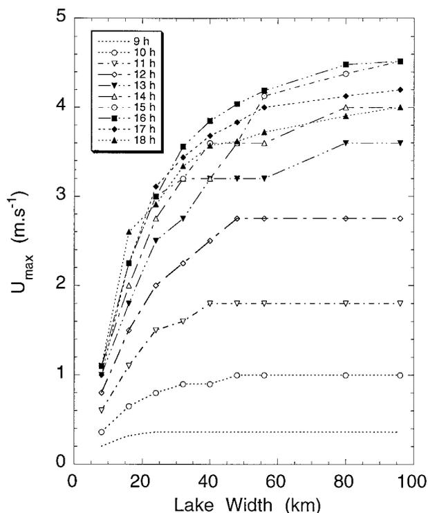
FIG. 2. Simulated maximum  $u$  component ( $u_{\max}$ ) of the LB (in the simulated vertical cross section) at various hours (as indicated) for 2D lakes of widths of 8, 16, 24, 32, 40, 48, 56, 80, and 95 km (indicated by the symbols on the curves).
