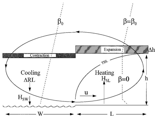
FIG. 1. Schematic illustration of features related to the scaling evaluation of the LB circulation (see the text for the notation). The air thermal expansion and contraction are magnified for purpose of illustration.
