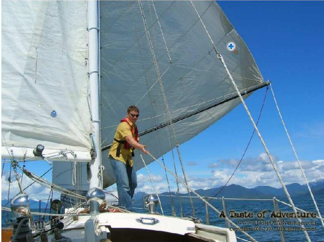
A whisker pole is better than a spinnaker pole since the former should be the length of the foot of the headsail and the latter is the J dimension (distance between mast and bow) of the boat. This can work really well especially if the wind is reasonably strong (>10 knots). Even in this approach, it is probably still not best to run directly downwind. Instead alternate between a broad reach (less wind) and a dead run (more wind) jibing as needed to make the most direct line to the mark.
