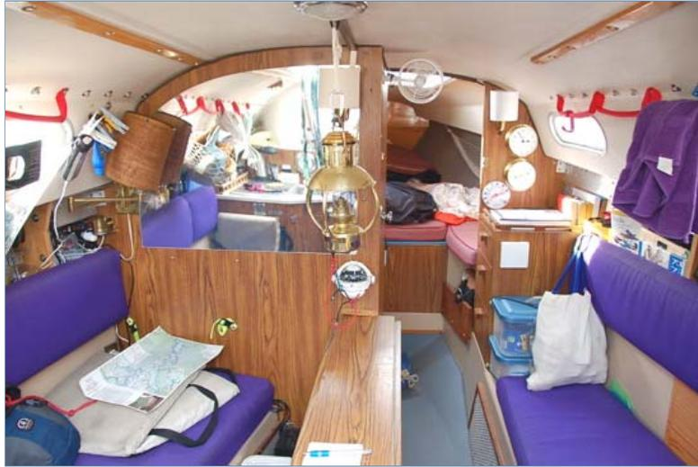
Looking forward: Windward's deckhouse extends almost to the bow, making for a roomy interior. The centerboard trunk, which Jeff has reinforced with Kevlar, supports the drop leaf table.
