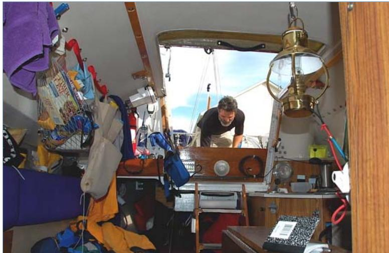
Looking aft is the galley. Under the cockpit, where the inboard would normally be found, is a large storage area. When not using sails, Jeff uses an outboard to push Windward.
